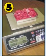
Press ENTER, automatically scale will count the pieces over the plate. If you require to count several closed packages, the scale features addition function, pressing this function will keep the sample and when you are done you will get
